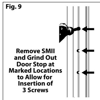
8. With the groove cut, you should now be able to easily slide the two pieces of the StrikeMaster II Pro into it's final install position. You will notice that (3) of the screw holes are now at least partially hidden behind the door stop. With a pencil, mark where those three holes are hidden on the door stop and remove StrikeMaster II Pro.
